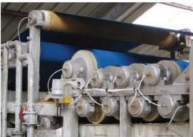
Food industry: lubrication of press ball bearings.
