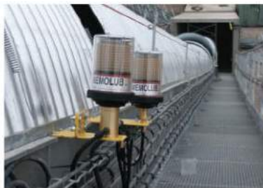
Mineral industry: lubrication of conveyor belt bearings.
