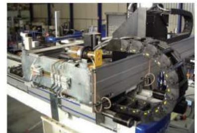
Robotics industry: lubrication of ball guides.
